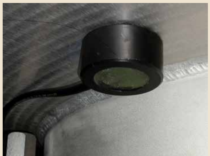
Fig. 1b The sensor is attached through adhesion directly onto the external surface of the tank bottom
